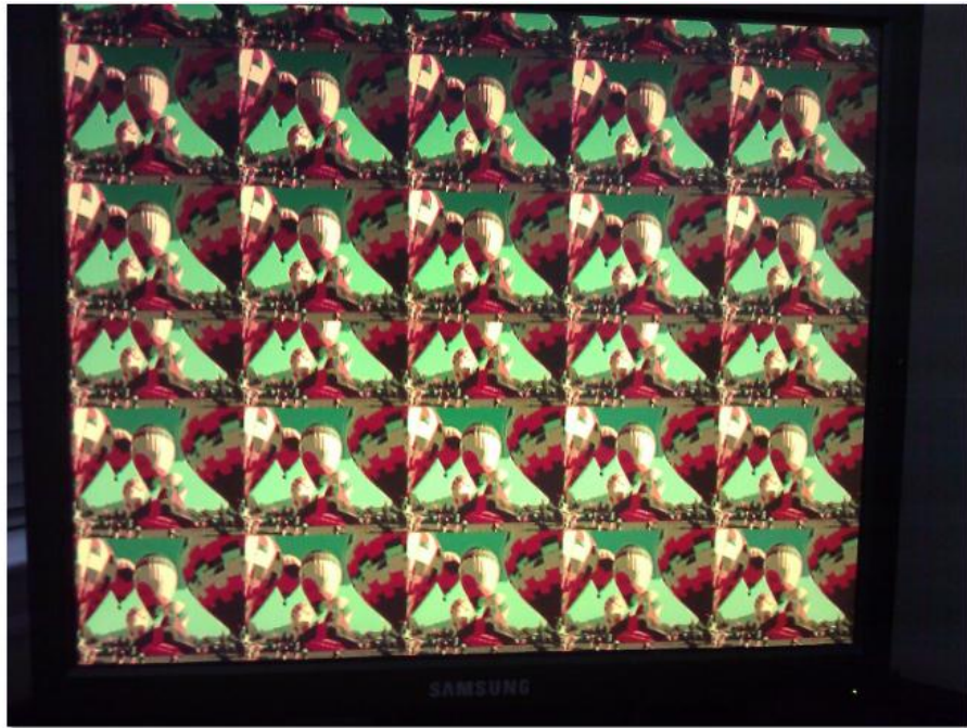
Figure 28: Close up of the Image displayed using the 16 bit custom VGA adapter
